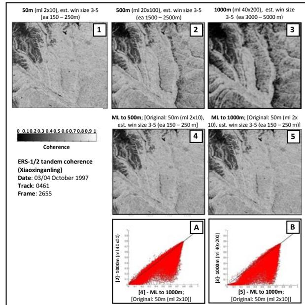
Figure 6. Interferometric SAR coherence variations of the two described estimation methods
